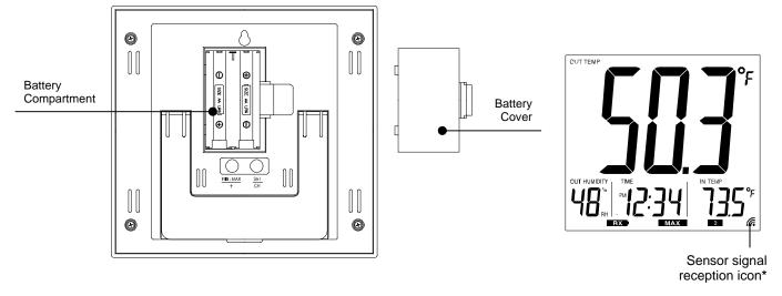
\* When the signal is successfully received by the Weather Station, the icon will be switched on. (If not successful, the icon will not be shown in LCD) So the user can easily see whether the last reception was successful (icon on) or not (icon off). On the other hand, the short blinking of the icon shows that a reception is being done now.
